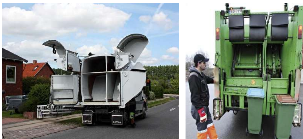
Figure 6 – Example of multi-chamber waste collection vehicles: a four-chambers vehicle on the left, a two-chambers vehicle on the right.
